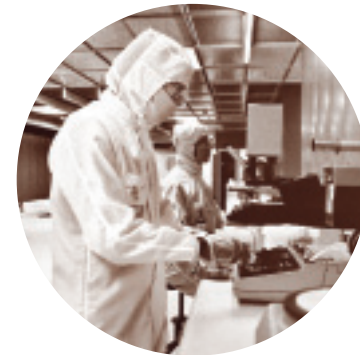
In Intel's factories, bunny suits replace smocks, to keep hairs, skin flakes, and other particles from falling on intricate circuitry.
