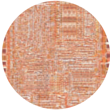
The 8080 microprocessor features 4,500 transistors and about ten times the performance of its predecessors.
